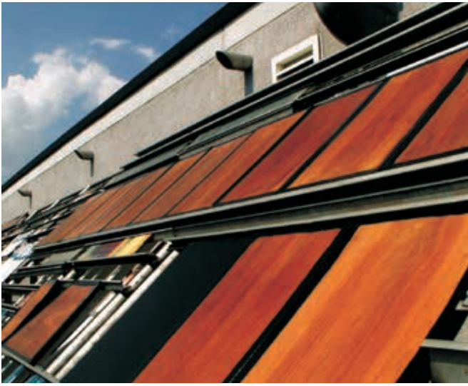
Figure 40 Outdoor weathering station of Evonik at the Wolfgang Industrial Park in Germany.
