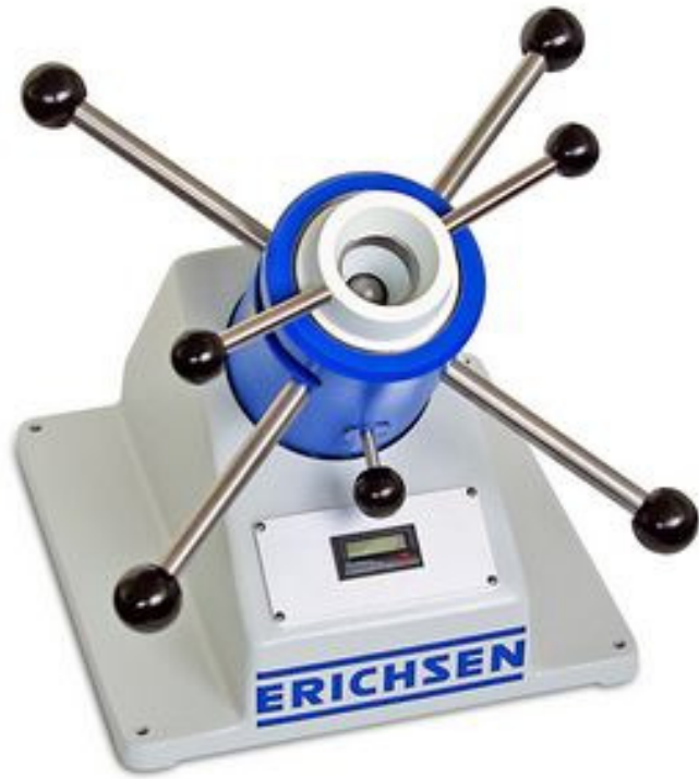
Tin-coated steel plate (200 μm): Tinplate rips @ 7 mm
